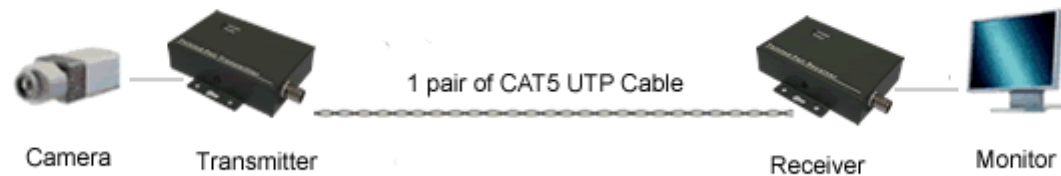
Active CAT5 Video Transceiver over 3000ft CAT5 Cable Video Transmission in CCTV system
